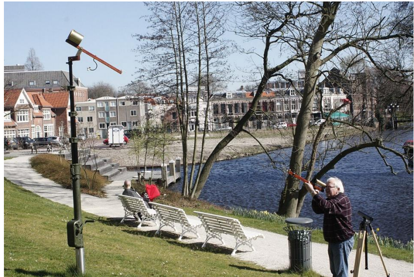
Figure 12 A modern recreation of Huygens Aerial Telescope Design
