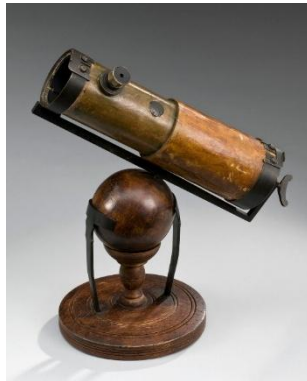
Figure 19 The first reflecting Telescope built by Sir Isaac Newton in 1668
